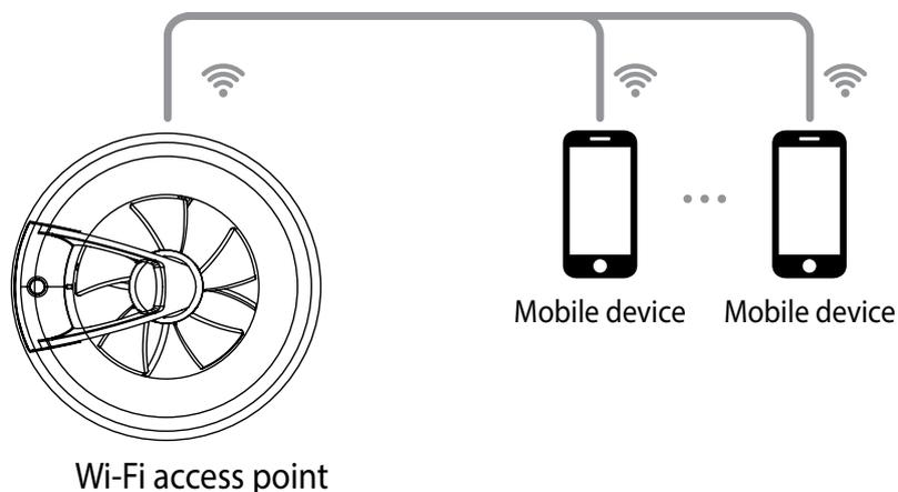
**Example 2:** Example 2: Connection diagram using a router with one Wi-Fi access point.
