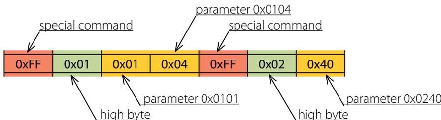
**The controller response (FUNC = 0x06) to the reading request**
