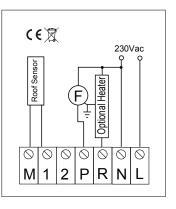
Fan: 2amps max Optional heater: 2amps max
