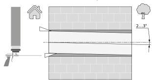
When installing the air duct, ensure that it is inclined towards the street.
