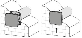
7. Install the outer ventilation hood or the grille.
