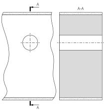
2. Install the air duct into the hole so that its cuts are aligned with the outside and inside surface of the wall. For ease of installation use the foam wedges included in the delivery.
