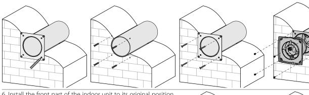
6. Install the front part of the indoor unit to its original position and fix it with a screw using a screwdriver.
